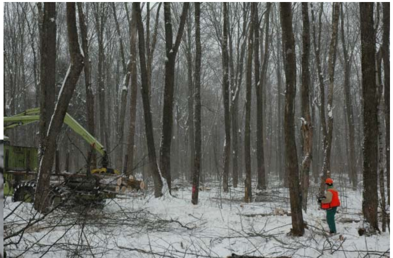
Technicians Dean Van Doren (above) and Joshua Kunzman (left) time logging equipment to determine timber harvesting costs and productivity.
