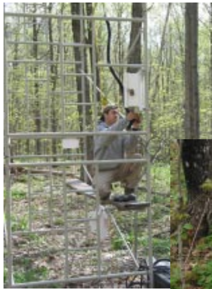
Field assistant Brad Herrick wires a datalogger affixed to a tower that will monitor above-canopy conditions (left). And later installs a below ground sensor (below).
